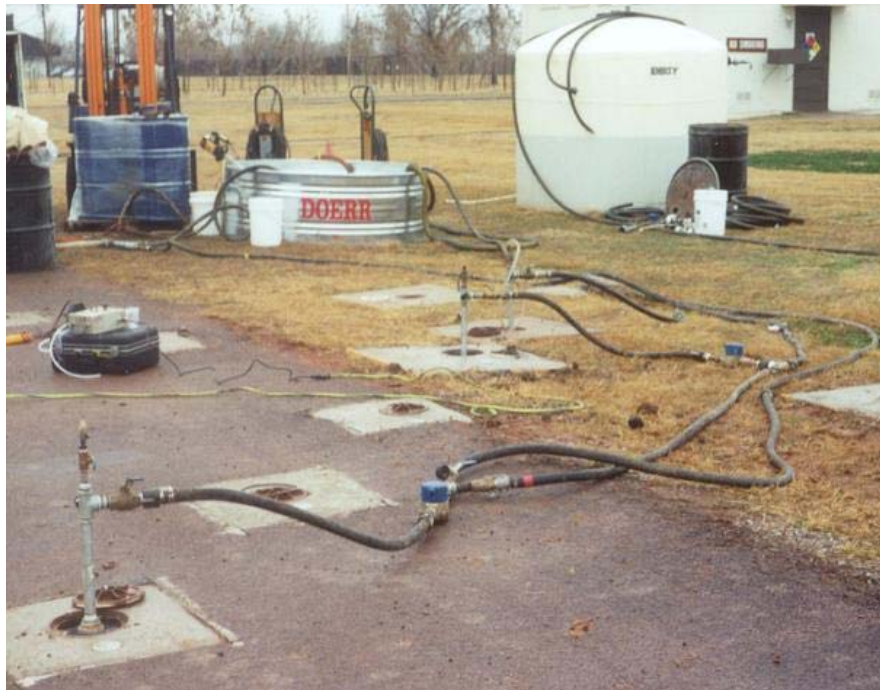
Figure 1.8 Typical Oil Emulsion Injection System Layout
